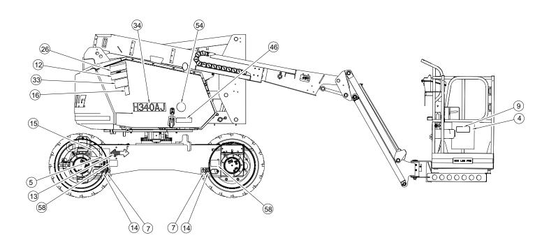
Figure 4-17. Decal Location - CSA - Sheet 4 of 6
