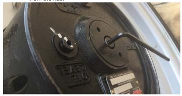
**3.** Locate the brake release bolts on the turntable and remove them. Install the cap retaining screws in the turntable in place of the brake release screws so they are not lost.
