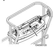
Cable is pressed, breaking the magnetic connection between the cable and right bracket.
