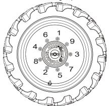
**3.** The tightening of the nuts should be done in stages. Following the recommended sequence, tighten nuts per wheel torque.
