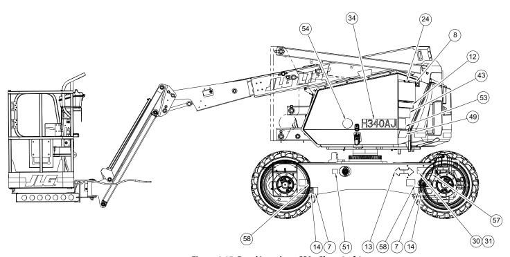
Figure 4-15. Decal Location - CSA - Sheet 2 of 6
