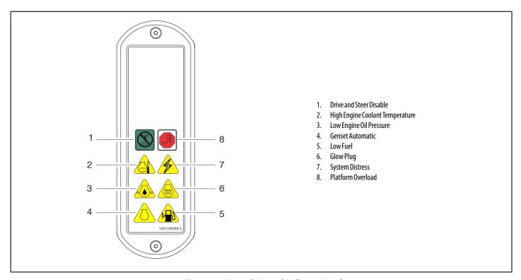
Figure 3-3. Ground Control Indicator Panel
