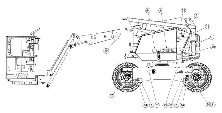
Figure 4-21. Decal Location - CE/AUS - Sheet 2of 6
