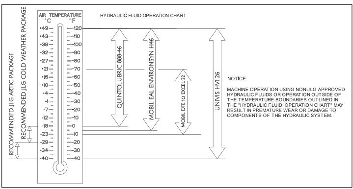
Figure 6-2. Hydraulic Oil Operation Chart - Sheet 1 of 2
