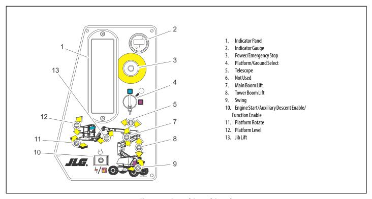
Figure 3-1. Ground Control Console
