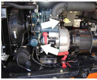
Lube Point(s) - Fill Cap/Spin-on Element Capacity - 2.6 Quarts (2.5 L) w/Filter Lube - EO
