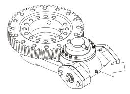
Lube Point(s) - Grease Fitting Capacity - A/R Lube - Mobil SHC 007 Interval - A/R
