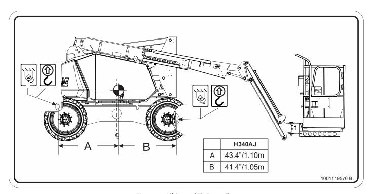
Figure 4-7. Lifting and Tie Down Chart
