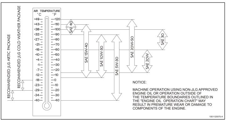
Figure 6-4. Engine Oil Operation Chart - Kubota
